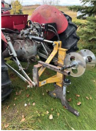
A homemade cable plow to pull the wire.
