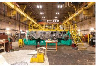
Esterhazy's mining machines are assembled in underground shops before being moved out into production areas to begin mining potash ore. Commissioning of a twelfth four-rotor mining machine began in January, and a thirteenth is expected to be complete later this year.
