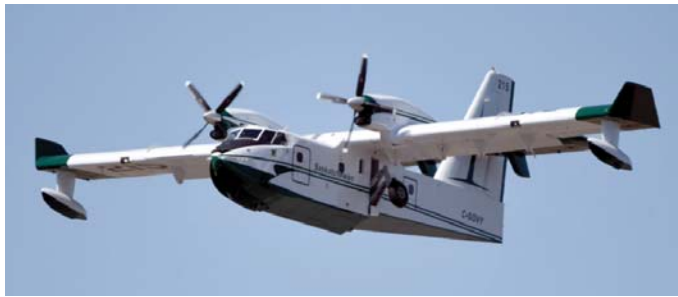
A CL-215T water scooping air tanker—one of six in the province's fleet—takes flight. Also part of the Saskatchewan aerial resources are four Convair 580A land-based tankers and seven smaller bird-dog aircraft.
