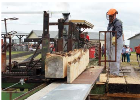
Lynn Tutthill operating the bush saw mill at the museum during Canada Day. The saw blade is operated by a pulley belt from a vintage steam engine tractor.
