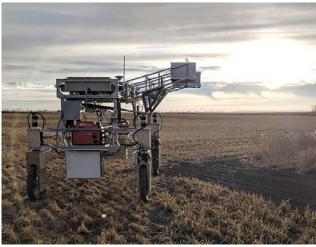
The Phenotype Acquisition and Measurement Machine (PAMM), a robotic imaging platform developed for field crop phenotyping, collects data on wheat, lentils and canola phenotypes.
