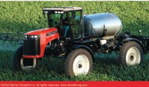
The new Versatile SX275 Self-Propelled Sprayer 1200 gallon tank MaxTorque mechanical drive Automatic transmission
