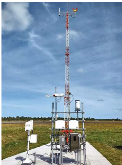
Right: The installation of an AWOS at Moosomin Airport will significantly improve aviation safety and accessibility.
