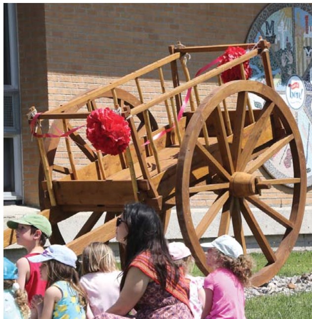
The Red River cart symbolizes a mode of transportation that Métis used to transport cargo to and from, the Red River Settlement all across the North West. The cart was built with no nails and was constructed solely with wood.
